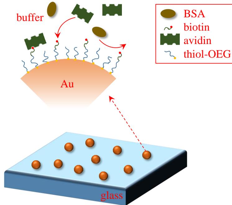
Figure 2. The biosensor design. Gold nanoparticles on a glass surface, functionalized with biotin, are used to capture avidin. The binding is detected through changes in the optical spectrum of the nanoparticles.
