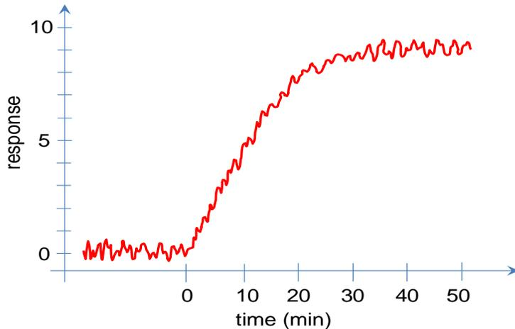
Using the information from the previous question, we have  $\Gamma$  after 10 min. Equilibrium corresponds to the final value which is about two times higher. Multiply with molecular weight to get mass coverage ( $0.68 \text{ ngcm}^{-2}$ ).
